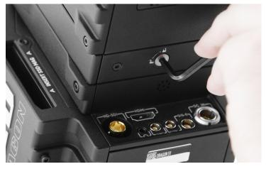
The Pro I/O Module is secured.
